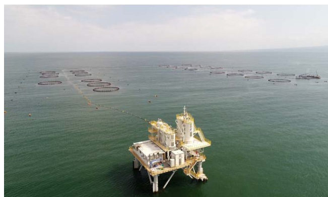
Platform-type automatic feeding system for large-scale off-shore fish farming (salmon) at Sakaiminato city, Tottori Prefecture Yumigahama Suisan Kaisha, Ltd.
