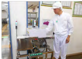
Machines that allow participants to experience what it feels like to be entangled in conveyor belts
