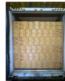
Stacking to Prevent Collapse
